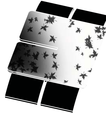
photoluminescent coating photoluminescent paint selected to reach full luminosity after 12 hours of light exposure. shadows from context during the day are imprinted, becoming visible at night
